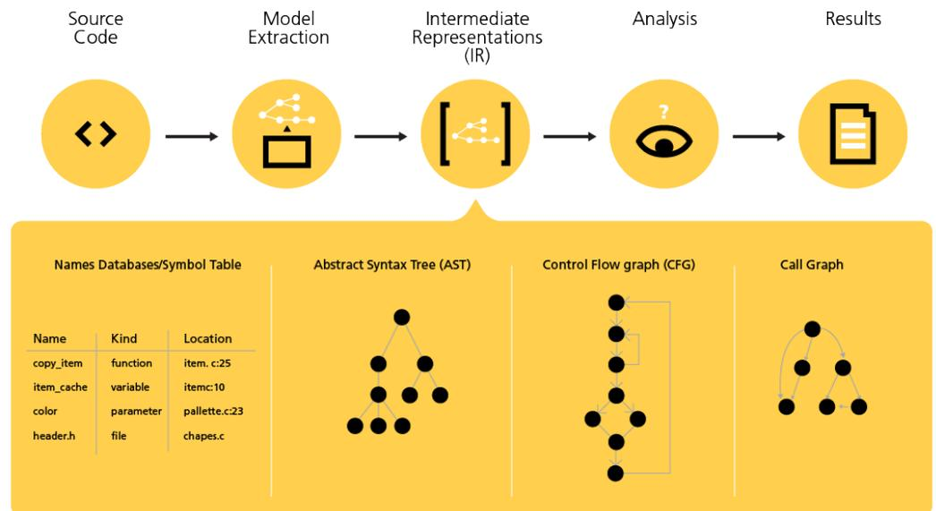
Figure 1. The architecture of an advanced static-analysis tool.
